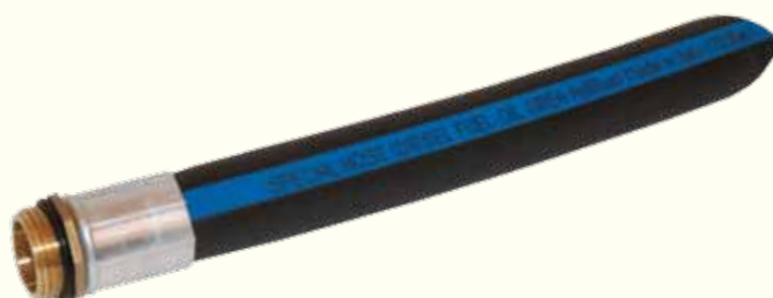
Mod. SP20/B Aluminium sleeves Hole: 20mm Int.Diam.: 28mm Ext.Diam.: 30mm For rubber hose mod. 902/SPEC20
