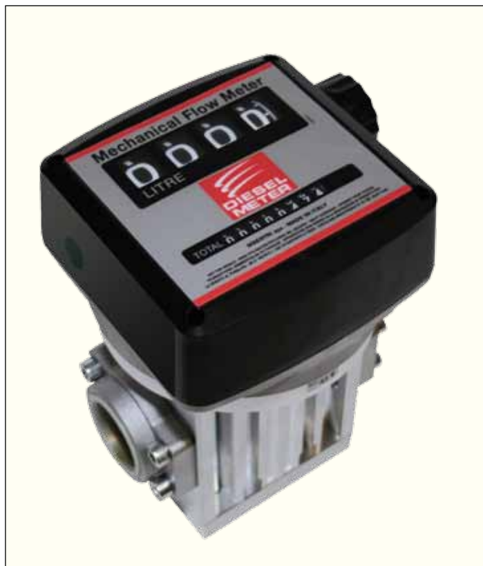
Mod. 804/MAXI “ MAXI ” Mechanical flow meter Flow rates: Min. 20 - Max 220LPM Inlet/Outlet: 1”-½BSP Female Precision: +/-1% - Weight: 5,8kg Dimensions: 181x155xh238mm Max pressure: 10bar - 140psi Bust pressure: 30bar - 420psi
