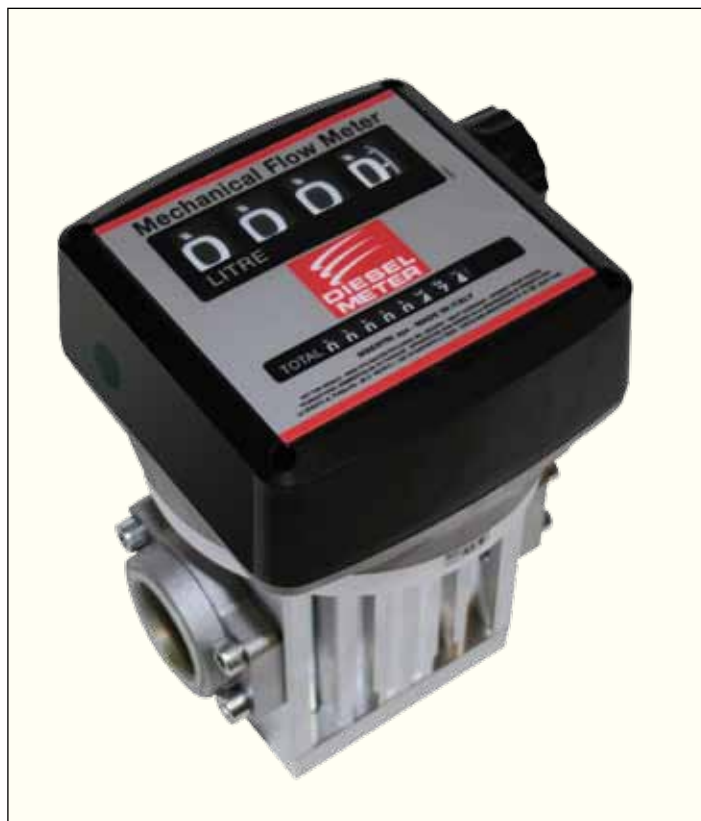
Mod. 804/MAXI “ MAXI ” Mechanical flow meter Flow rates: Min. 20 - Max 220LPM Inlet/Outlet: 1”-½BSP Female Precision: +/-1% - Weight: 5,8kg Dimensions: 181x155xh238mm Max pressure: 10bar - 140psi Bost pressure: 30bar - 420psi
