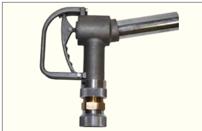
Mod. 709/M280 “ MAXI ” Manual fuel nozzle with swivel connector Inlet: 1”-½F - Max flow rate: 280LPM. Weight: 1.95kg - Terminal spout: Ø est. 45mm
