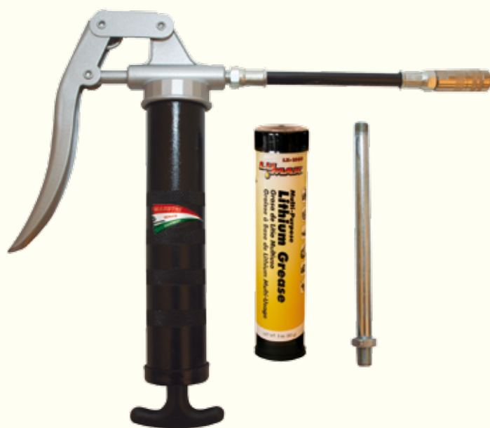
Mod. 116 Manual grease gun kit 85g Cartridges refill only (not for manual refill) • 85g Cartridge • 300mm flexible hose • Rigid pipe • 4Jaw fittings Max pressure: 200 atm Flow rate: 60g/min (0,6g/strike)
