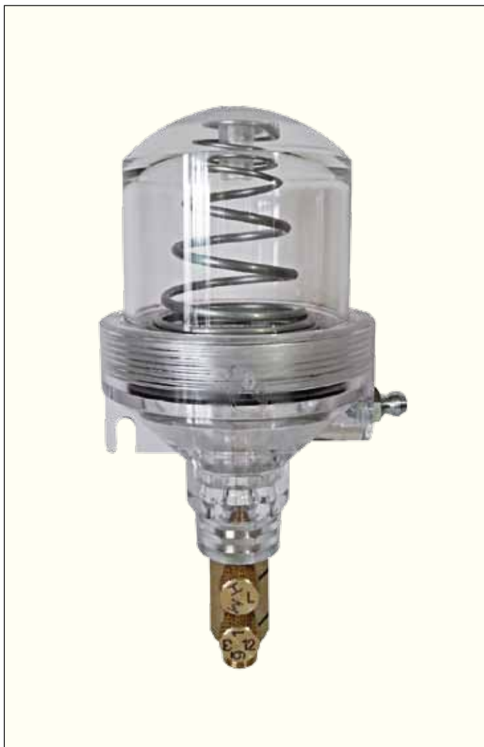
Mod. 595/A100 AUTOMATIC LUBRICATORS MANUAL REFILL Capacity: 100cc High: 135mm - max diameter: 77mm Thread: 10X1M
