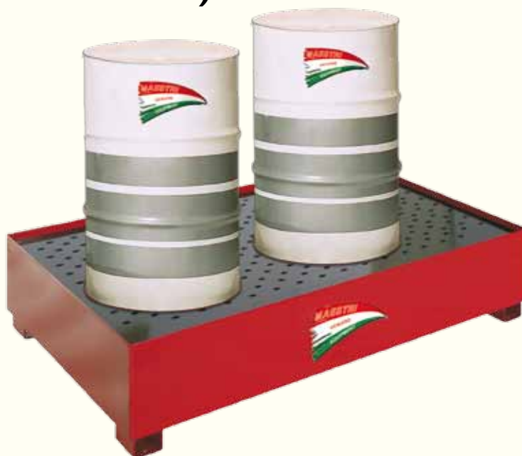
Mod. BASE 2 Metal base base for two 200kg DRUMS Capacity: 286L - Measures: 135x83x34cm Weight: 55Kg
