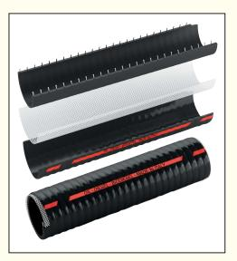
Two-layer hose in thermoplastic PVC, PU, NITRILE RUBBER compound with embedded galvanised steel spiral with polyester yarn reinforcement for suction and delivery of oils, diesel and bio diesel.
