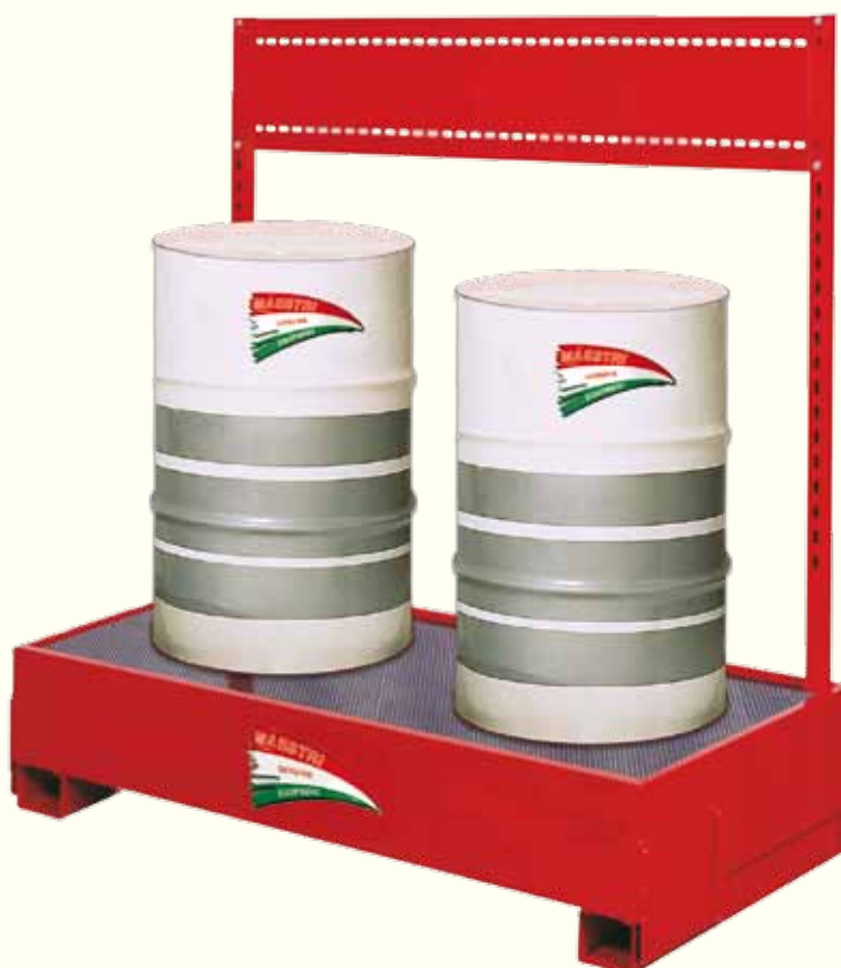
Mod. BASE 2 COMP Metal base for two 200kg DRUMS with drilled steel plate and posts Capacity: 286L - Measures: 135x83x230cm Weight: 95Kg
